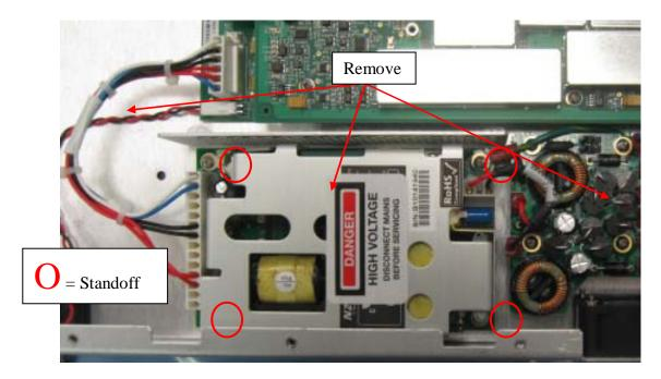
5. Install new AC power supply (PS-0000075), power harness (CA/WR12831-1), new ground cables (PL/6140-4 & PL/6140), insulator cover paper (FP/8393-1), high voltage label (LB/DNGR-HV40X28) and AC input filter (PL/10105-1). See pictures below.
