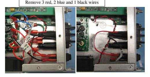
3. Remove the two (2) mounting screws and ground lug nuts. Remove the DC input and install the AC input (PF-0000001). Install two (2) fuses (FS-0000032) into the fuse housing.
